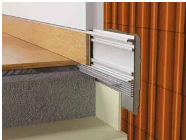
BFZ is a construction profile that allows you to create a flush-to-the-wall baseboard with the same material as the flooring. In the lower part there are special grooves, designed to allow the insertion of a linear profile which will help to determine the level of the screed and ensure perfect positioning of the heights of doors and windows.
